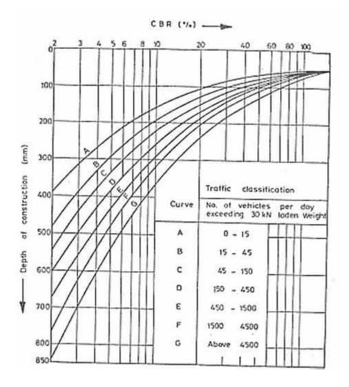
Fig -2 IRC design chart for flexible pavement design
