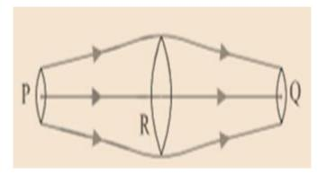
We will be able to determine the boundaries the selected points in the plane by the same set of the streamlines. Hence, the particles of fluid passing through the surfaces at the three-point P, R and Q will be the same. Now consider the area at the three points as  $A_P$ ,  $A_R$ , and  $A_O$ . Consider the speed of the fluid particles as  $v_P$ ,  $v_R$ , and  $v_q$ .
