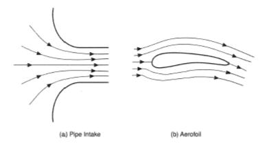
Streamline flow in fluids is defined as the flow in which the fluids flow in parallel layers such that there is no disruption or intermixing of the layers and at a given point, the velocity of each fluid particle passing by remains constant with time.
