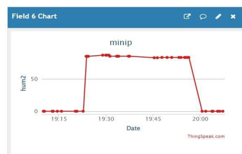
Figure 3.5: Humidity Levels Over Time(Node2)
