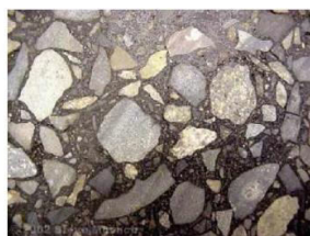
Fig. 2.1 Dense graded HMA surface
