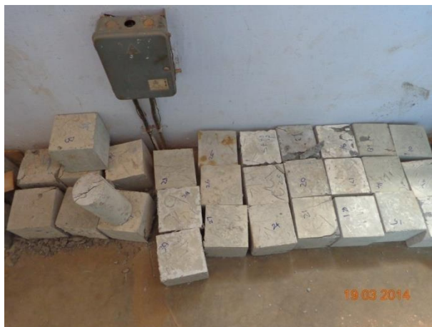
Tested cubes & cylinders
