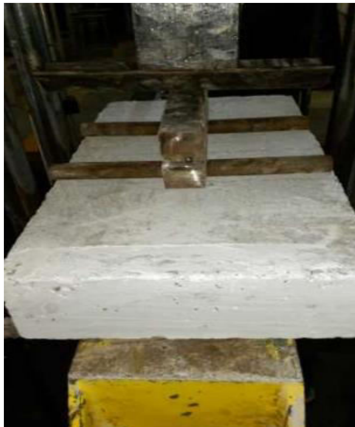
[Fig.4.4: Two point load test setup]
