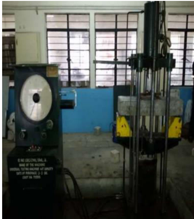
[Fig.4.3: Universal Testing machine (40 ton capacity)]
