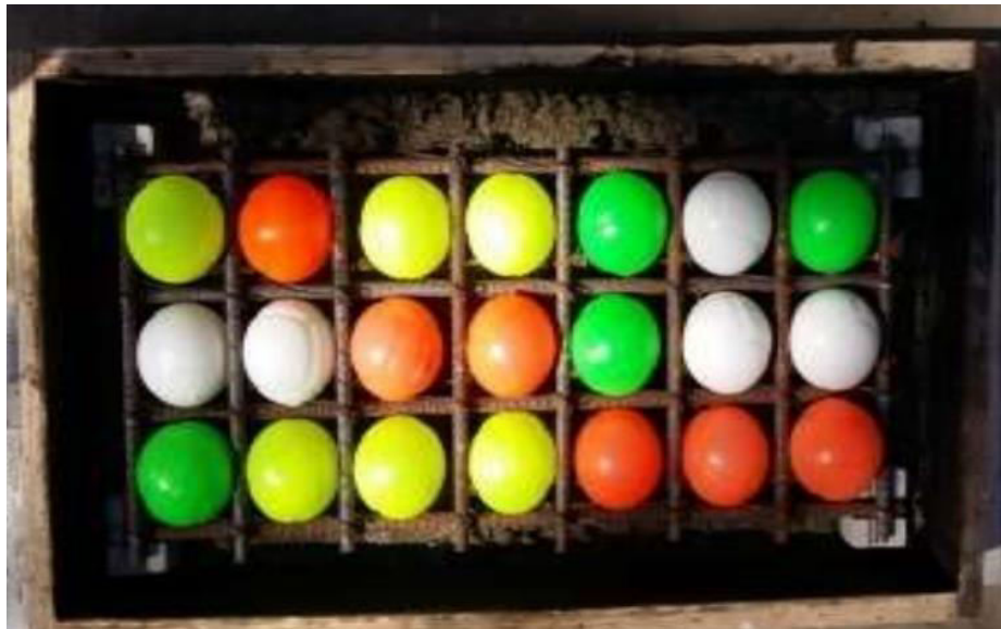
[Fig.4.1: 60 mm diameter ball arranged at 20 mm spacing in a slab of size 600mm*300mm*100mm]
