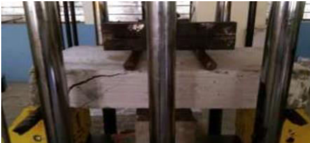
[Fig.5.2: Shear crack in specimen BD 8 of slab thickness 100 mm]
