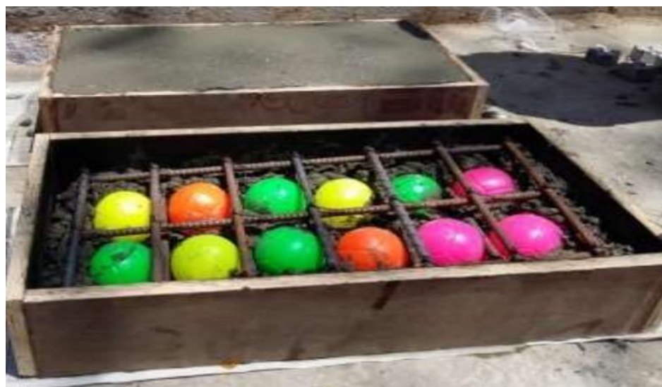
[Fig.4.2: 75 mm diameter ball arranged at 20 mm spacing in a slab of size 600mm*300mm*100mm]
