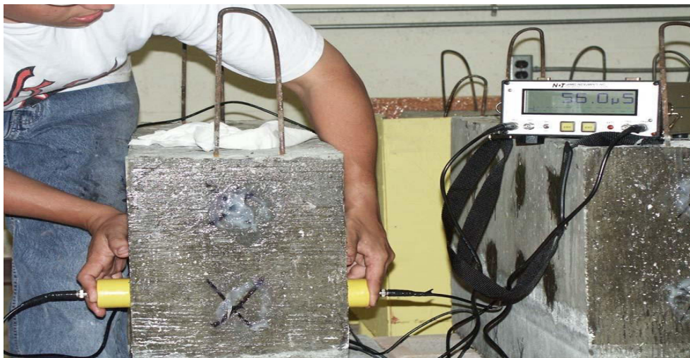
Fig.USPVTTester used for testingofabeam
