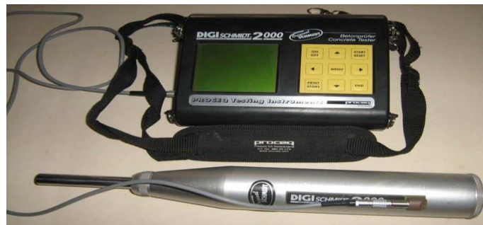
Fig. Rebound-HammerComponentsare usedin Project
