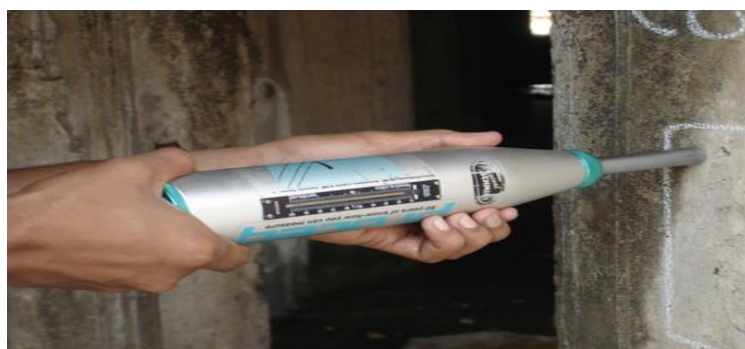
Fig. Specimen testing of Rebound-Hammer
