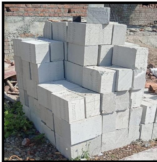
[Fig.4.4: AAC blocks of sizes 0.6 \times 0.19 \times 0.15 m]
