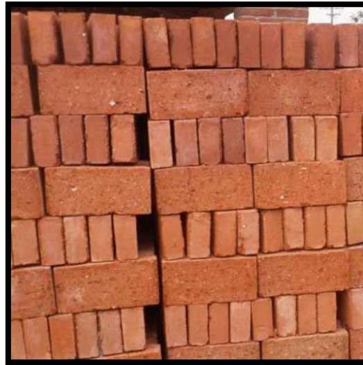
[Fig.4.3: Collection three conventional bricks of size 0.19 \times 0.09 \times 0.09 m]
