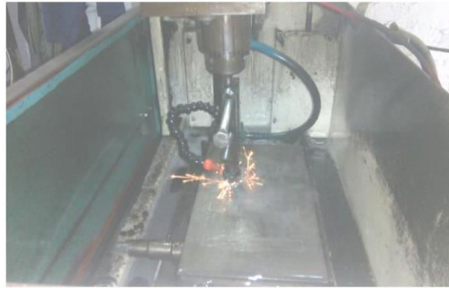
Figure 8: Generation of spark during EDM operation.
