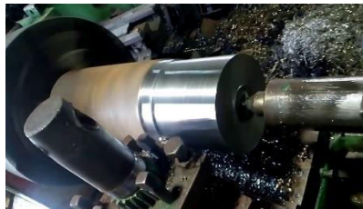
Figure.5: Turning operation on lathe machine
