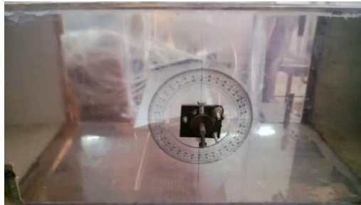
Figure 3: Airfoil Model Mounted in Tunnel Test Section
