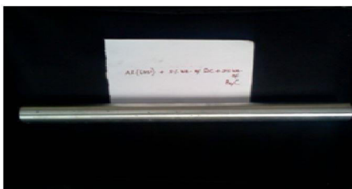
Figure 4.1 Al (6351) + 5 wt. % of SiC +5 wt. % of B 4 C
