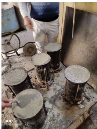
Fig. 3: Sample preparation for Split Tensile Strength
