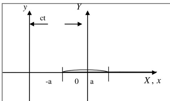
**Fig.1:** Dynamic punch on elastic half-plane situated on a line segment.
