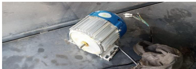
Fig. Motor [750 watt and 2800-3500RPM]
