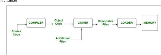
**4.2. Loader:** It is special program that takes input of executable files from linker, loads it to main memory, and prepares this code for execution by computer. Loader allocates memory space to program. Even it settles down symbolic reference between objects. It is in charge of loading programs and libraries in operating system. The embedded computer systems don't have loaders. In them, code is executed through ROM. There are following various loading schemes:
