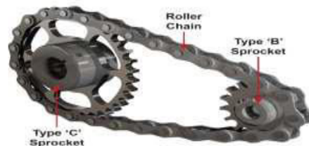
Fig. VI .8.1 Chain and sprocket [11]
